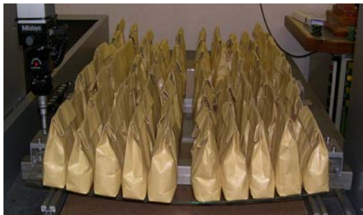
Fig. 3: Photo of laboratory test setup at ECN to verify and validate laminate bending predicted by FEA
