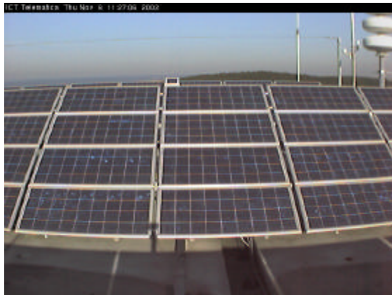
Fig 2: Test setup at ECN in Petten (The Netherlands). Every minute the lower 9 pv-modules are connected in shunt and in string, and a photograph is taken. A 1000 points power versus voltage sweep takes 7 seconds
