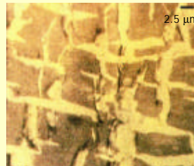
Aluminium-oxide layer crushed under the high pressure of a contact force. The darker areas are oxide, the lighter metallic aluminium
