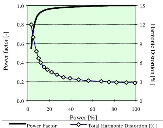
Figure 2. Power factor and total harmonic distortion OKE4
