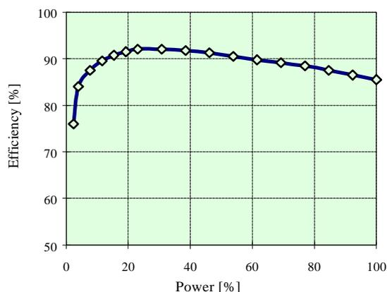
Figure 3. Efficiency of OKE4
