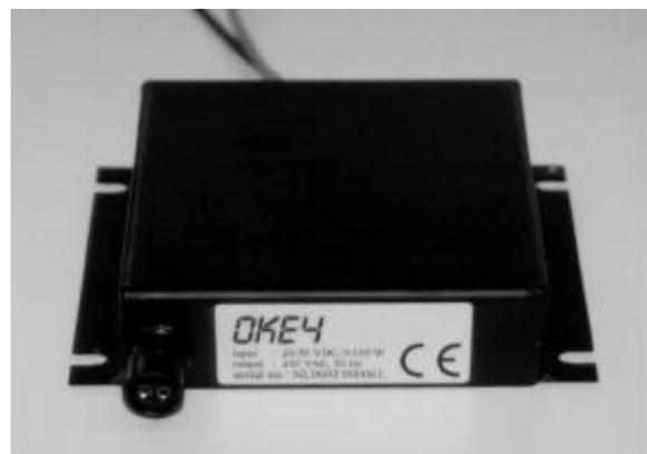
Figure 1. OKE4 inverter
